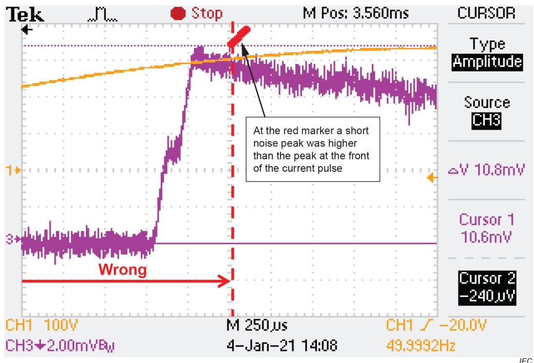
Figure 1 – Incorrect measurement
