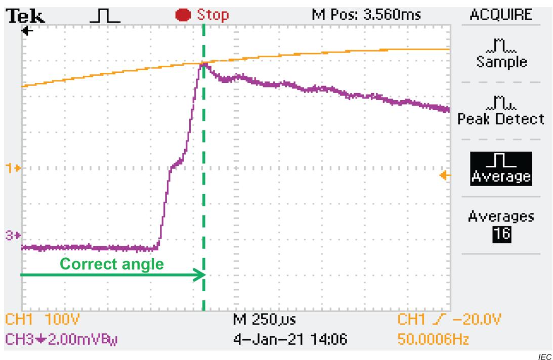
Figure 2 – Correct measurement with averaged waveform
